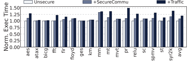
Fig. 11: Execution times when secure communication and security metadata are cumulatively considered, normalized to the unsecure 4-GPU system.
