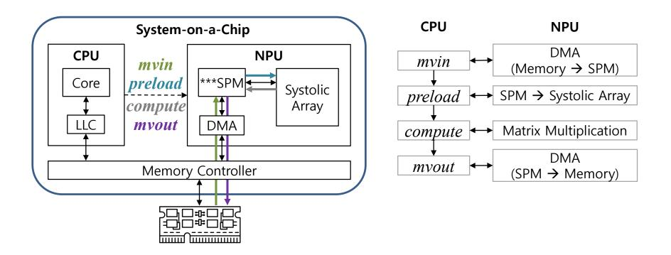
\*mvin: move-in, \*\*mvout: move-out, \*\*\*SPM: Scratchpad Memory
